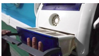
7. Slide the filter tray along the groove
