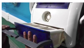
7. Skyv filterplaten tilbake i bassengroboten langs sporet
