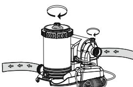
**IMPORTANT: DO NOT DRY RUN THE FILTER PUMP** – Make sure both the pool's Inlet and Outlet valves are fully covered by water before operating the Filter Pump.
