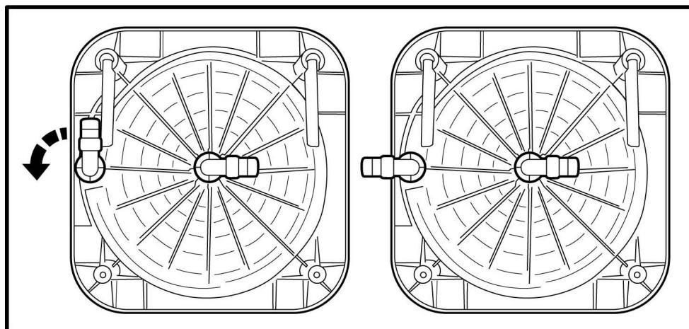
To detach the hose connectors from the main base, turn the connectors clockwise until it stops and then pull it away.
