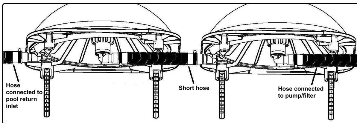
For connection of 3 or more heaters, it requires a 3-way valve (not included) and "T" connector (not included) to be installed. Below is an example of above ground pool with 3-way valve set up in place.
