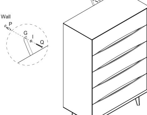
Fasten the safety strap to your wall using appropriate fixings for your wall type. If you are unsure, please seek professional advice on how to attach this safety strap to your specific wall.
