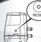
If the pump is not heating properly, please press the thermal cut-out manual "Reset" button on the pump.
