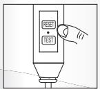
The PRCD plug must be tested before each use to avoid risk of electric shock. Do not use the pump if this test fails.
