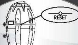
If the pump not heating properly, please press the thermal cut-out manual "Reset" button on the pump.
