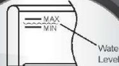
Fill the water level between maximum and minimum printed on the SPA wall.
