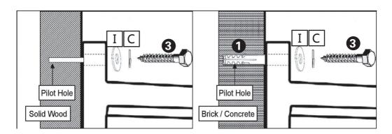
**Solid Wood:** Drill 1/8" pilot hole at all four marks. Thread M10 lag bolt through lock washer, M10 flat washer, and wall mount bracket and into each pilot hole. **Solid Brick/Concrete:** Drill 7/16" pilot hole at all four marks. Tap wall anchors into each hole with hammer. Thread M10 lag bolt through lock washer, M10 flat washer, and wall mount bracket and into each pilot hole. Tighten securely.
