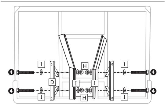
Attach the wall mount brackets (D) with V-bracket (E) by using four bolts (4) and eight washers (I) with four lock nuts (H).
